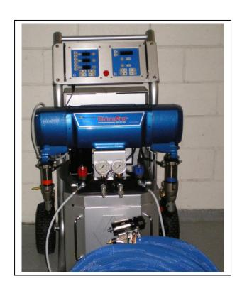
Max Output: 11 kg/min @ spray tip Max operating Pressure: 3500psi
