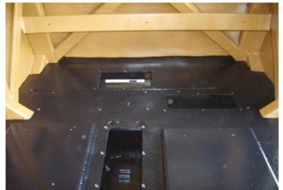
The job was completed over a three day period using a 1/4" fine texture atomizer. The extremely fast cure time of Rhino Tuff Stuff, allowed easy application to vertical and overhead surfaces.
