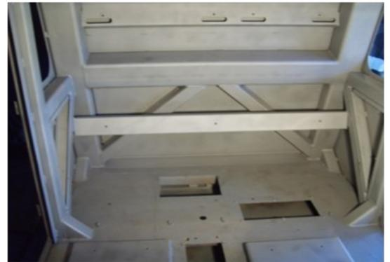
The cab was first sandblasted and repaired prior to application of Rhino Prime 251. It was then sprayed with Rhino Tuff Stuff. The Rhino Tuff Stuff was applied to the cab at a nominal thickness of 2mm to the inside roof, walls and console, 4mm to the underside of the cab and to the inside of the doors and the floor. The floor also had non slip particles applied.
