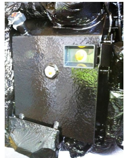
Hydraulic Tank Coating
