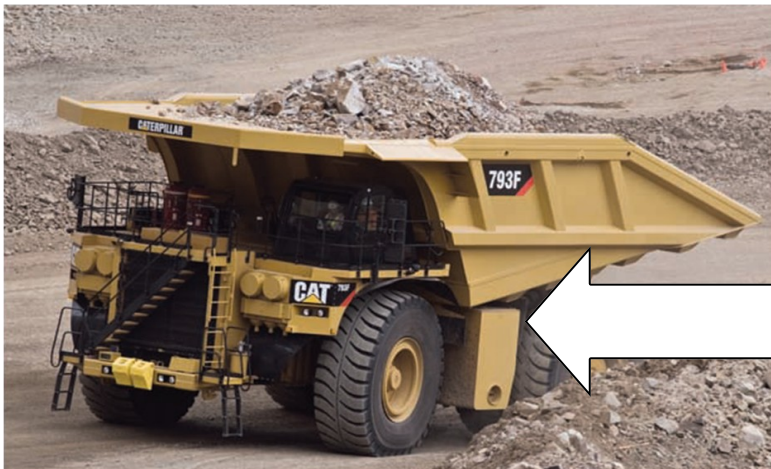
Left: This picture of a CAT 793 shows the position of the fuel tank.
