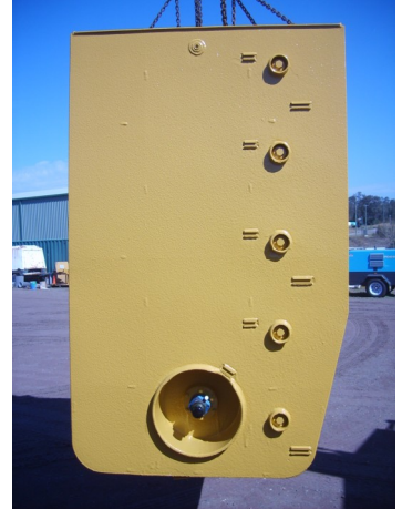
Above and Below: The completed fuel tank after Rhino and painting Caterpillar yellow
